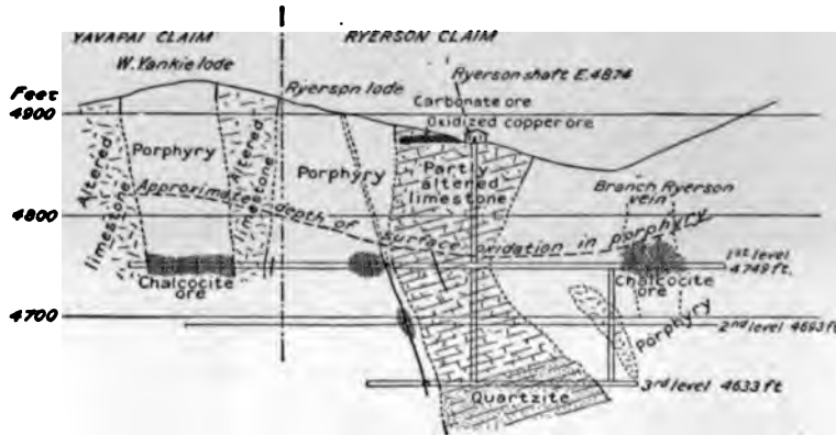
FIG. 123. — VERTICAL SECTION, RYERSON SHAFT, MORENCI. (LINDGREN)
